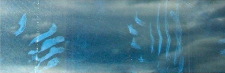
**Figure 6.** A portion of a thermal/double-pane window after a hole had been made in it. Images occurred because during the assembly of the mirror by a worker with no gloves left handprint and fingerprint deposits that interacted with a silver monolayer surface, making the handprints from the window assembly visible.
