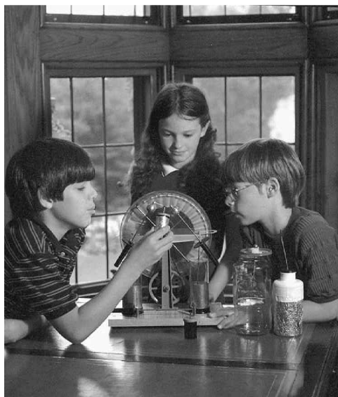
Fig. 8. The children are examining a Wimshurst static-electricity generator and some charge-storage devices, one of them a facsimile Leyden jar using foil to collect charge.
