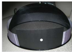
Energy collector with 1 cm white dot as target
