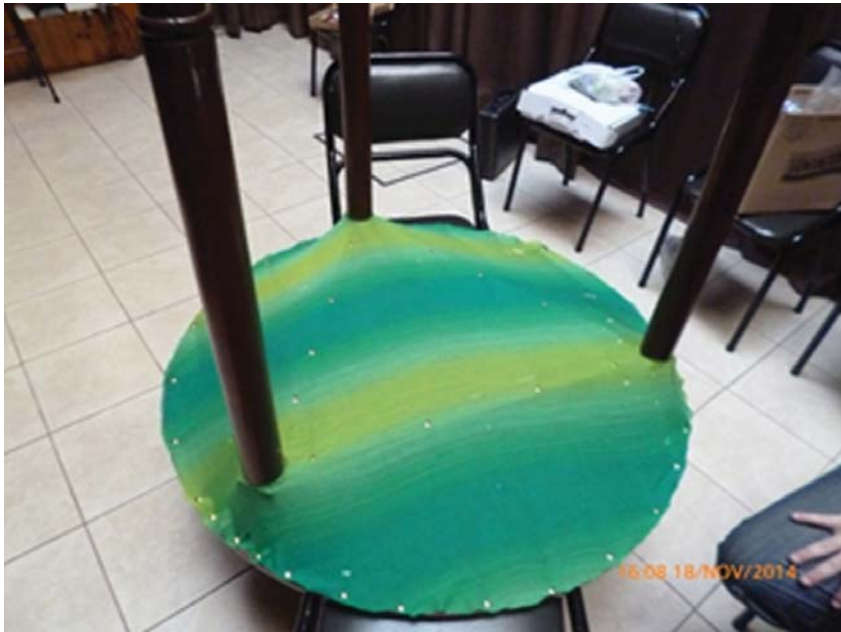
Photo 2. The piece of fabric had been nailed to the undersurface of the table, ready for the foam.
