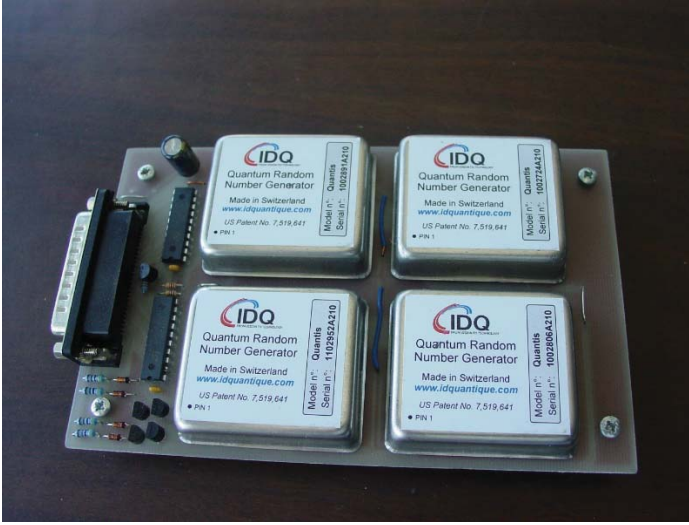
Figure 4. The REG source for the replication machine.
