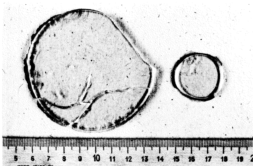
Fig. 1. Photo of round glass pieces that fell out of window glass during thunderstorms
