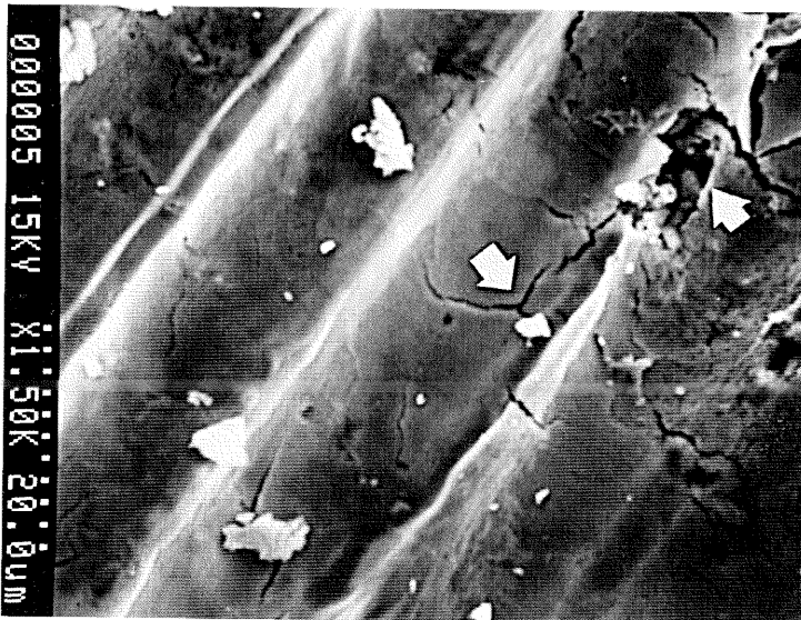
(3b) Scanning electron microscope (SEM) view of plant contacting surface of coating, showing region at right arrow where heated gasses escaping from a stomate apparently blew a hole in the film. Central arrow indicates a type of crack pattern typical of a rapidly cooling glaze film (1500X).
